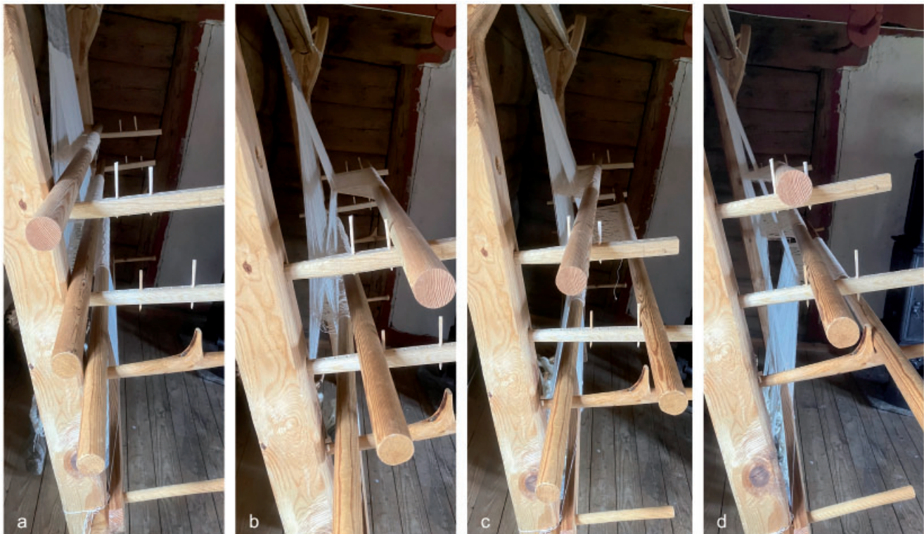
Fig. 7: Placement of the heddle rods to form the four 2/2 twill sheds, using double-notched supports for the upper two support pairs: a) shed 0 is open, all heddle rods at rest against the uprights; b) shed 1 is open, heddle rod I in outer notches; c) shed 2 is open, heddle rod I in inner notches and heddle rod II in outer notches; and d) shed 3 is open, heddle rods I and II in inner notches and heddle rod III in single notches (Images: Katherine Larson)
