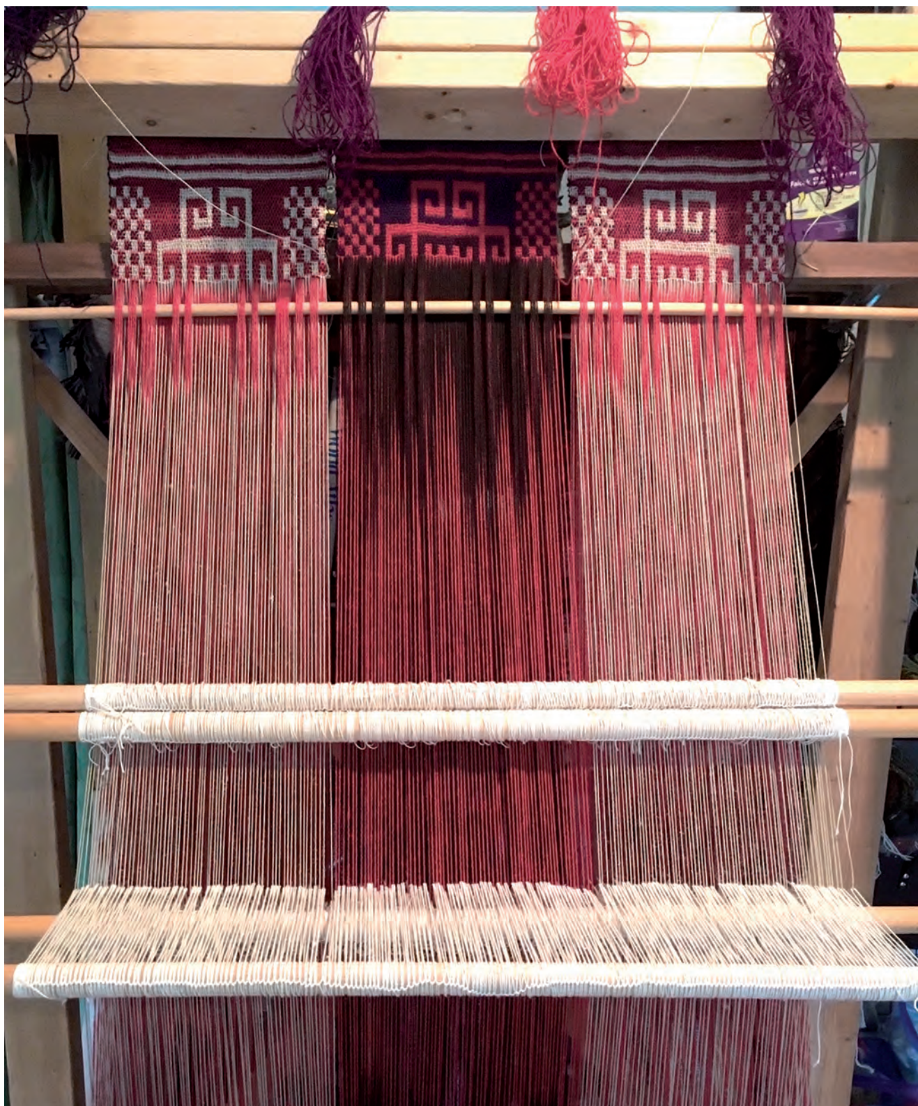
Fig. 7: Fibre-test warp with a forward-layer weaving shed open (third heddle). Note layer separation close to the pattern stick below the fell: sections with linen-layer warp threads (left and right) cleared opposing-layer warps slightly better than in the blended wool/hair section (centre); observation of errant warps in both left and right sections of this shed: none; in centre section: several (Image: Katherine Larson)
