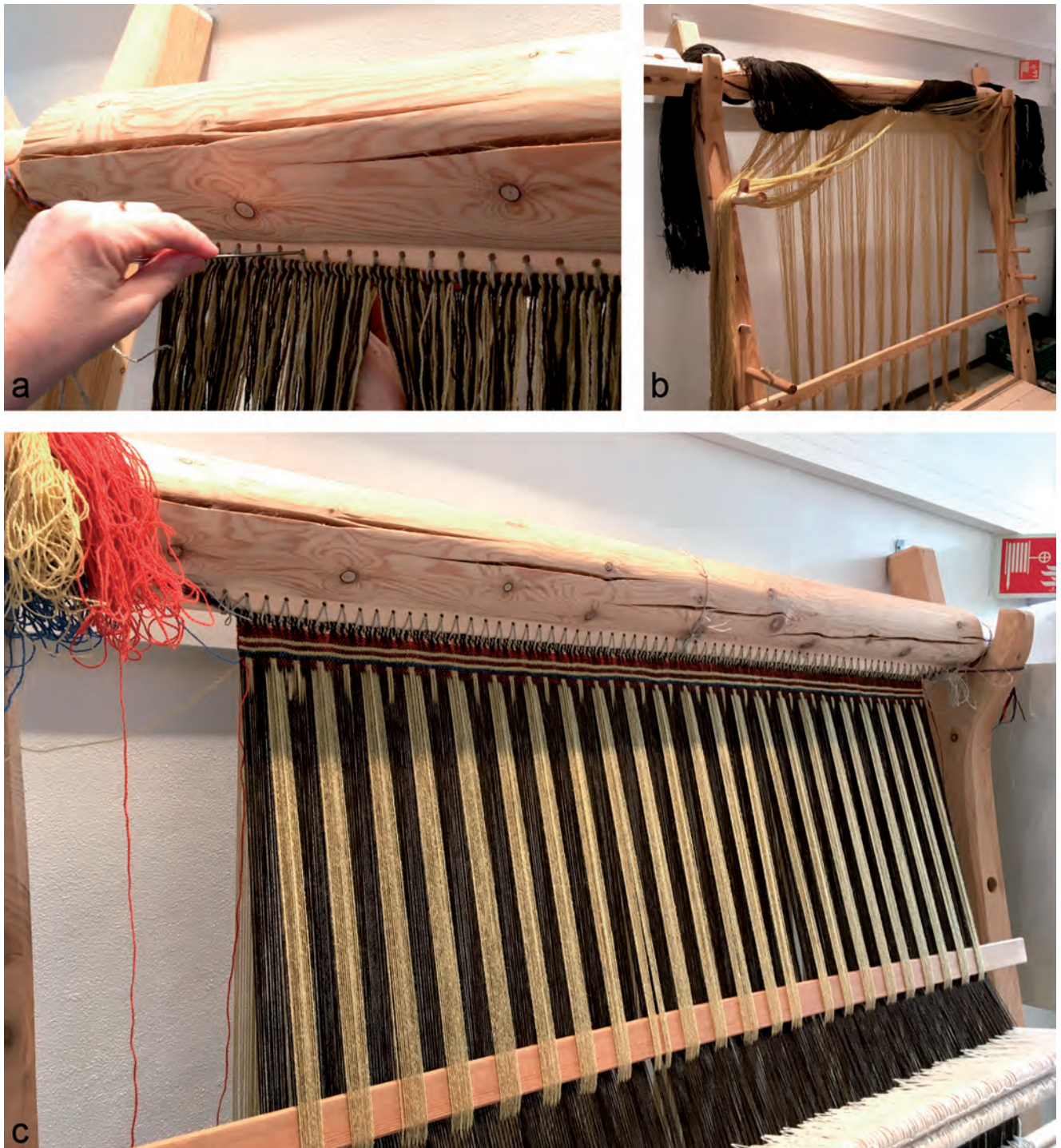
Fig. 3: Establishing the coverlet-width warp at Osterøy Museum: a – sewing the warp to the beam; b – separating warp threads to apply the first row of weights and spacing chain; and c – beginning pattern weaving (Images: Katherine Larson)
